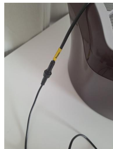
Figure 10 – Sensor power cable connected to the 12 VDC supply, with the locknut tightened.
