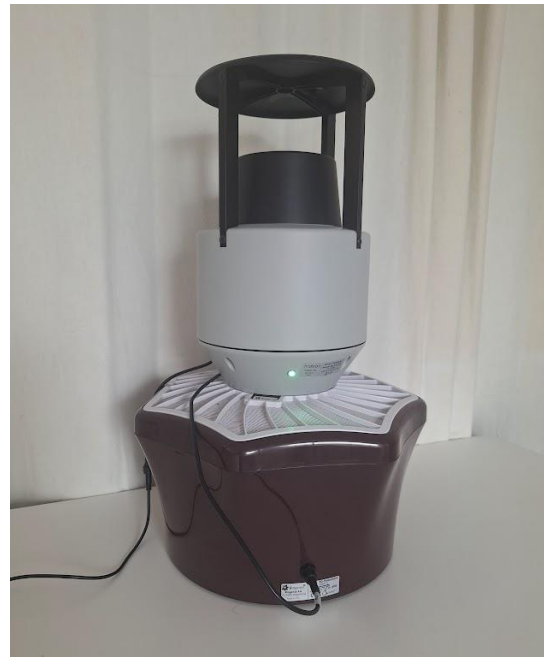
Figure 11 – Vectrack sensor mounted on a trap, with the Power and Trap cables connected.
