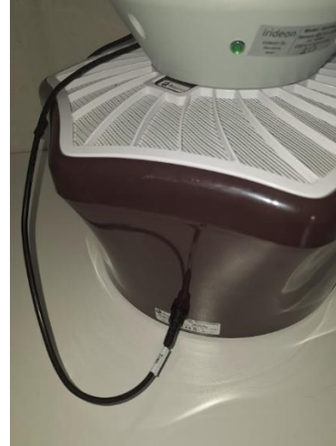
Figure 8 – Sensor trap cable fitted, with the locknut tightened.
