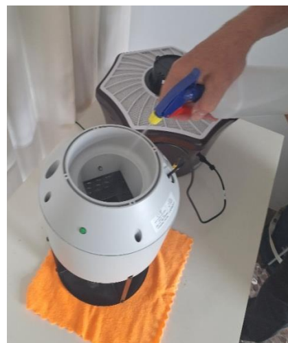
Figure 12 – Spray the solution onto the walls of the flight tube.
